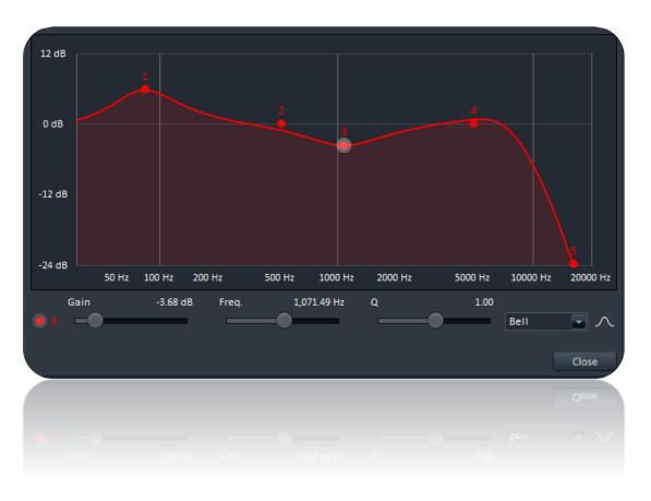
Click on a red dot to adjust the parameters of the corresponding band: gain in dB, center/cutoff frequency in Hz, Q factor, as well as the type of filter: bell, lowshelf, highshelf, lowpass or highpass.
